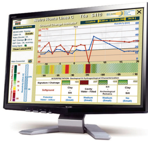
Fig.3 BEAM INTEGRAL interface; Forecast results represent a water-filled cavity of about 2m width in 4m ahead of the TBM.
